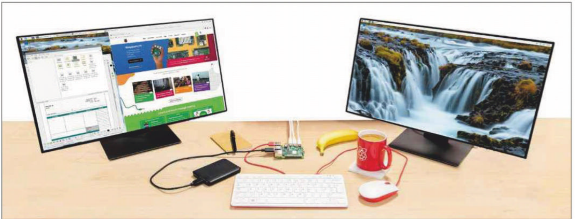
The Raspberry Pi 4 has two HDMI Micro ports, so you can set it up to use two screens simultaneously
